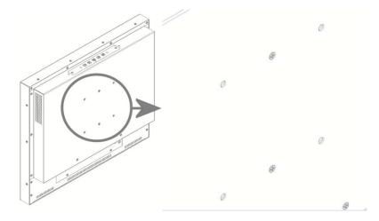
The desktop models can be mounted on any mounting bracket or pedestal corresponding with the right VESA mounting interface standard. Please refer to the dimensional drawings in this manual. Use M4 screws, max insert in the monitor is 8mm.
